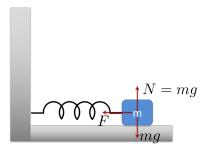
Consider the small oscillation of a mass attached to a massless spring on a frictionless surface. The one degree of freedom is x – the position of the mass. The mass experiences three forces: the gravitational force mg which is balanced by the supporting force from the surface N = mg and the restoring force from the spring F. Therefore, the motion x(t) of the mass is only affected by the
