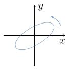
every z point in the wave, the electric field traces out the same oval shape, but with a phase shift from one point to another.
